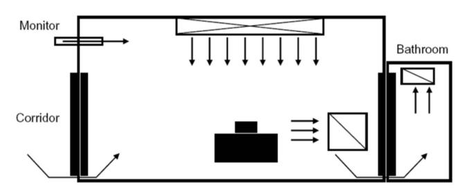
Standard AIIR without ante-room: Stacked black boxes represent patient's bed. Long open box with cross-hatch represents supply air. Open boxes with single, diagonal slashes represent air exhaust registers. Arrows indicate direction of air flow. Illustration from Guidelines for Environmental Infection Control in Healthcare Facilities, Centers for Disease Control, 2003.
